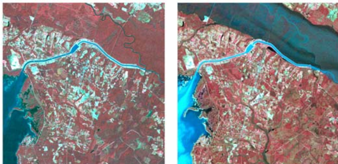
Impact of Hurricane Hugo on the land cover of the Francis Marion National Forest, South Carolina. Left Landsat-TM image was taken on 10/14/1987 and right image on 10/11/1989 (displayed using Bands 4,3,2). Hugo struck South Carolina on 09/25/1989. (Lam, Kulkani, and Zhou, 2004)
